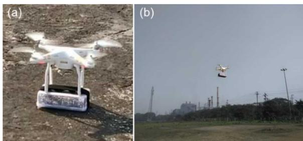
**Figure 3.** Placement of the air quality (a) monitoring system on the UAV and (b) monitoring of air pollutants in industrial zone at 5 m above ground level.
